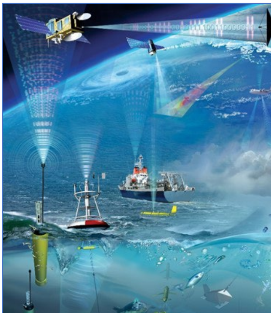
Figure 5: Ocean observing systems utilize satellites, radar arrays, weather buoys, survey vessels, and autonomous and remotely operated vehicles to collect data needed to understand how seasonal and long term cycles may be changing. Artwork by Glynn Gorrick.
